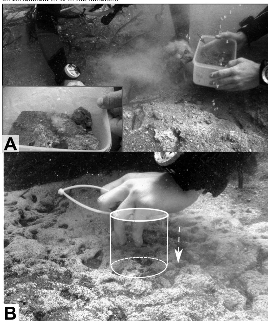
**Fig. 2:** Two tested sampling methods in La Calcara. **A:** Sampling of softrock material with a PVC-Box (4.2 L). The material decomposed under air pressure. Degassing structures stay stable under water (small picture in frame). **B:** A transparent cylinder was vertically inserted into the softrock underground to sample degassing structures (redrawn schematically with white lines). After sampling the opening was covered with a small board.
