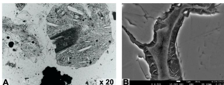
**Fig. 1:** **A:** Transmitted light capture of a decomposed mineral (hydrothermal alteration) with a magnification of 20. This outer shape of the minerals is common in the sample material. **B:** FeS<sub>2</sub>-mineral with small interstices which contain small (?fecal) pellets (scale: 1 µm).
